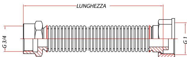
**sitecont® protex** is a flexible austenitic stainless steel hose covered by a protective and insulating polyolefine sheathing, for gas counter connections.
